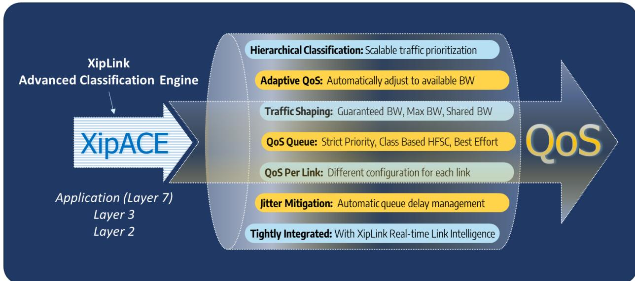
Any XipOS instance can also tag, mark or re-mark specific traffic as it leaves the device. This enables the network operator to deliver an end-to-end integrated QoS system using differentiated user classes or queues. This capability can be used to prioritize some traffic or limit the bandwidth used by others.
