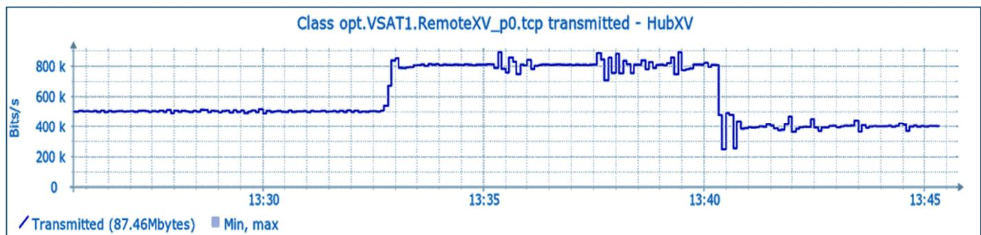
**No retransmissions are observed:** When the estimated bandwidth changes there are no retransmissions due to how the well-integrated TCP acceleration is seamlessly adjusted in concert with the overall QoS (as described earlier):
