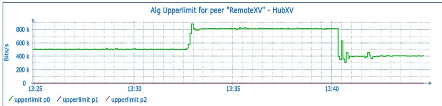
**Traffic transmitted onto the link:** Transmitted traffic very closely tracks the estimated capacity of the wireless link.
